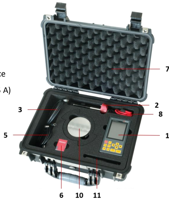
Fig. 1: Case with content (Pos. 4, 9, 12 not visible)
