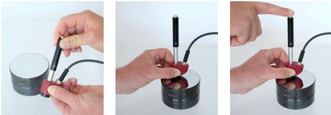
Fig. 13: Test with impact device type D
