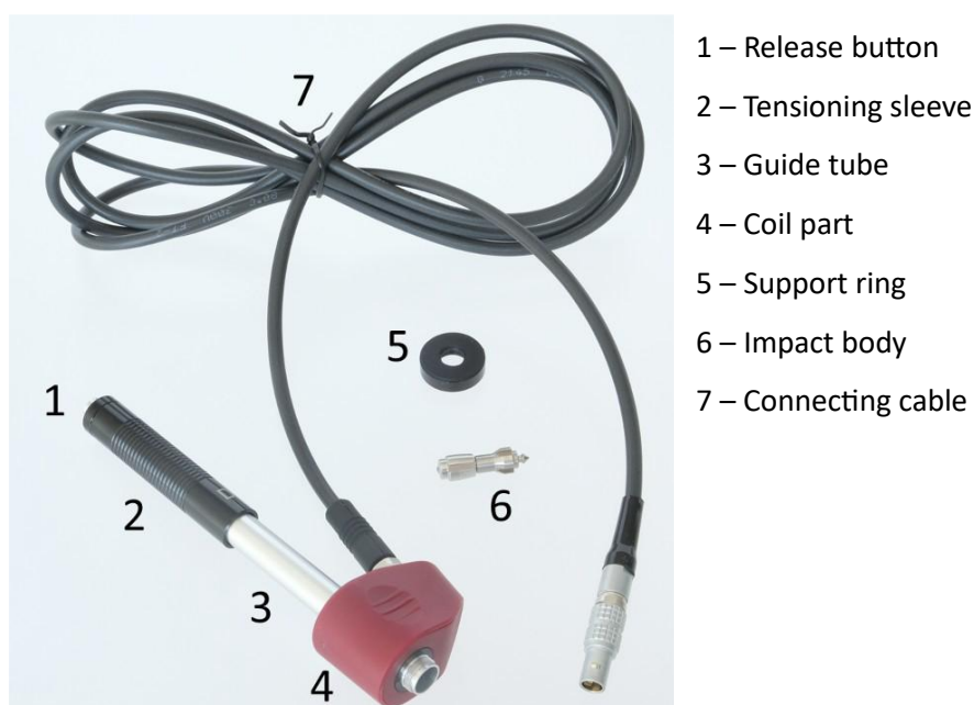
Fig. 12: Components of impact device type D
